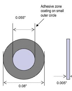
Required filter dimension (Drawing 18x actual size)
